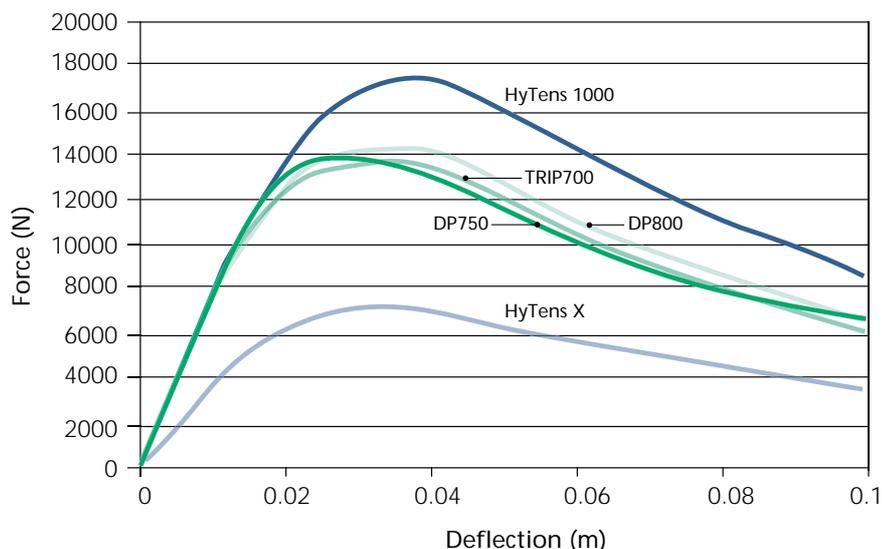
**Figure 8:** Force-displacement curves from the quasi-static impact test for the five different materials.
