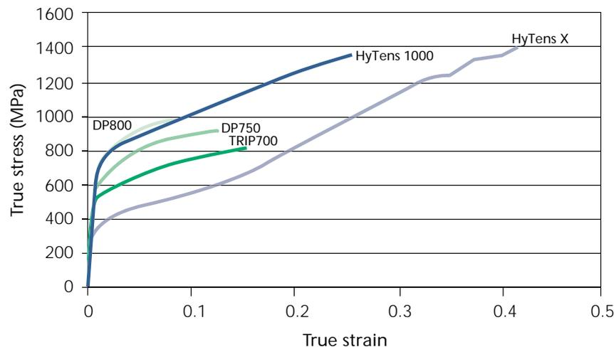
Figure 2: The true stress-strain curves up to maximum tensile strength for the materials in this study.
