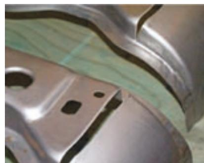
Fig 5. The fracture on the bumpers made with DP800.
