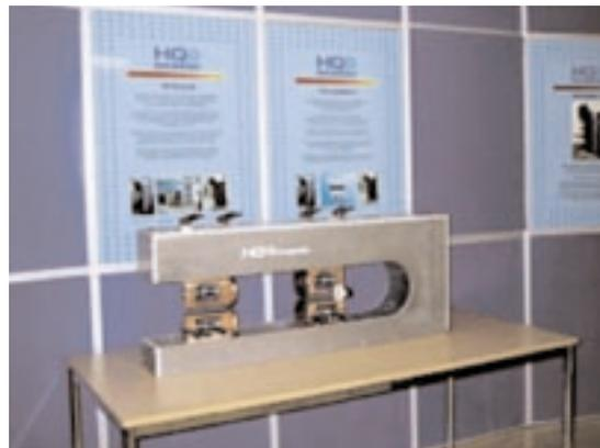
Fig 6. The BlancForm technique utilised for bending and a prototype machine for blank preparation of bending lines.
