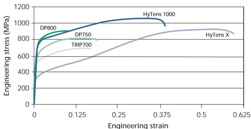
Figure 1: The engineering stress-strain curves for the materials in this study.
