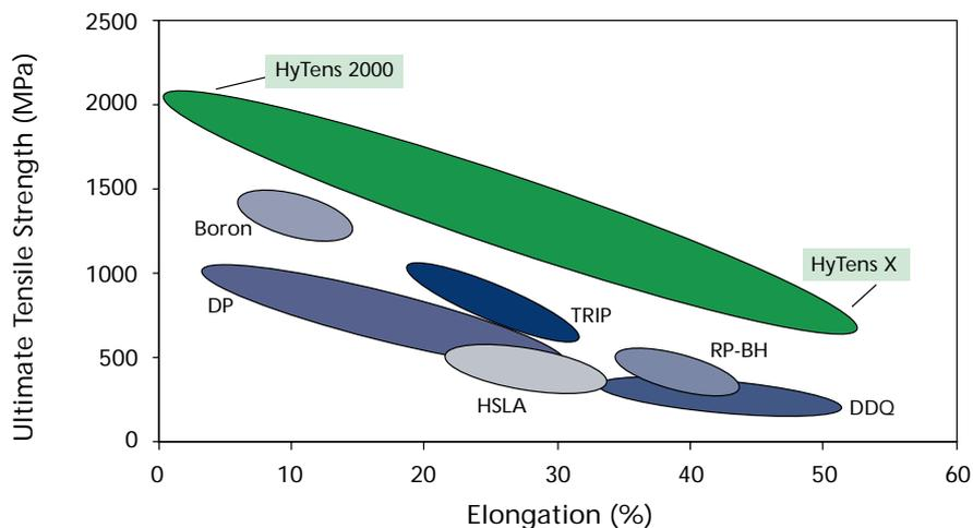
Fig 2. Strength-ductility combination for HyTens in comparison to carbon steel grades (DP = dual phase steel, TRIP = complex phase steel, HSLA = micro-alloyed steel, RP-BH = rephosphorised steel with bake hardening, DDQ = deep drawing grades).
