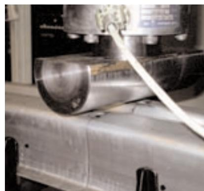
Fig 6. The configuration used to test the energy absorbing capabilities of a rear bumper.
