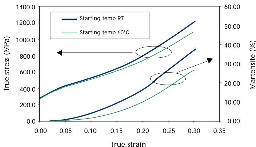
Fig 3. Stress-strain curves for HyTens X with differing specimen temperatures (25°C or 60°C).
